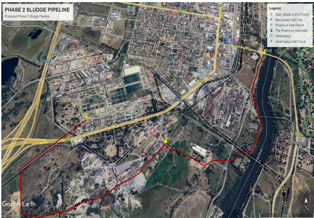
Figure 2: Aerial Map of the Phase 2 Sludge Pipeline.
